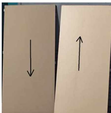
Improper Assembling for Metallic Colours
