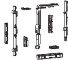
ÇİFT AÇILIM KİLİTLEME MEKANİZMA TILT AND TURN BASE MECHANISM
